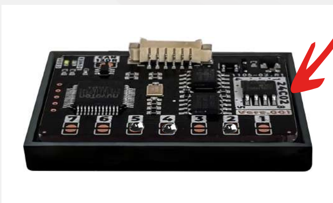
Please Remove The Original Eeprom and Insert the Eeprom into the Emulator
